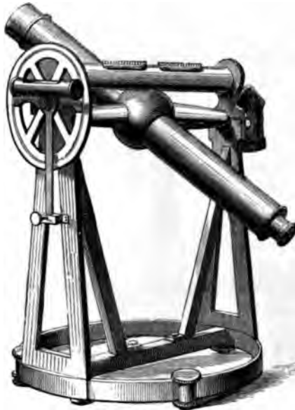
THE PORTABLE TRANSIT INSTRUMENT.
